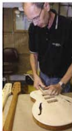
Above: Dantzig tests the neck fit on a Monaco III
